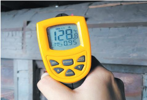
*Insulation of Tea Withering machine does not function well.*
