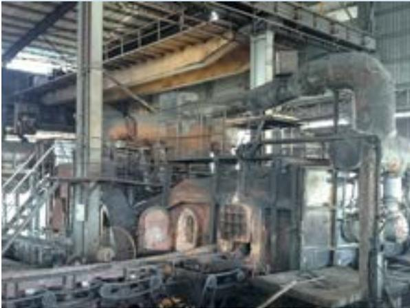
*Reheating furnace in steel processing*
