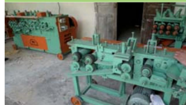
Nua bamboo splitting machine, sanding machine, and grinding machine in L&amp;V company
